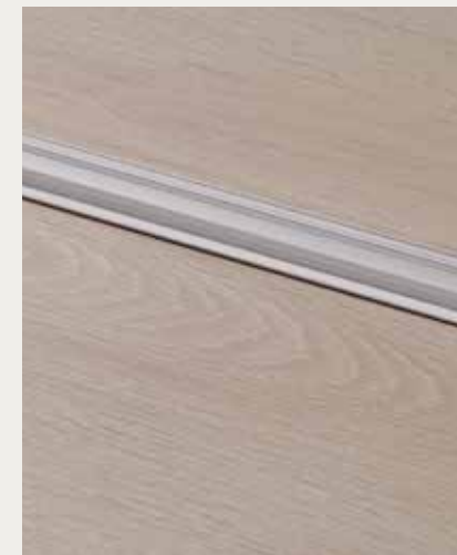
MULTIFUNCTIONAL PROFILE SILVER 1860 × 47 × 16 mm The Pergo multifunctional profile can level height differences for a smooth transition on to any other type of floor. Suitable for height differences of 0 – 12,3 mm. Surface: aluminium. PGPRSILV
